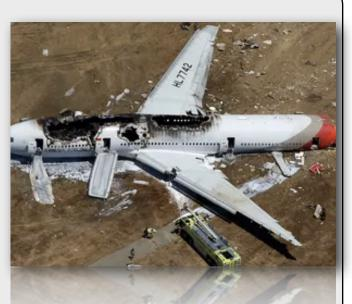
to the accident. Materials provided to airlines by Boeing that fail to make clear under what conditions the auto-throttle doesn't automatically maintain speed were also faulted.
